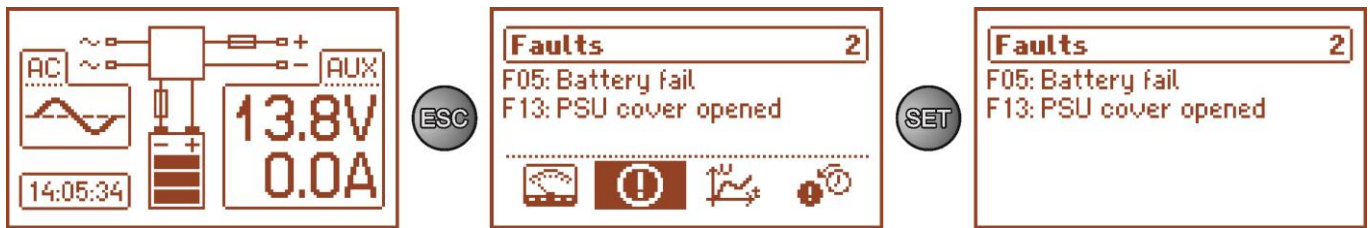
Fig. 10. LCD screen – current failures of the PSU.
