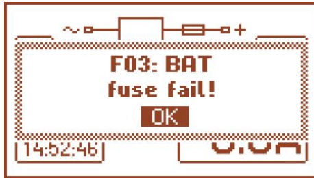
Fig. 9. Message indicating blown fuse at the AUX output.
